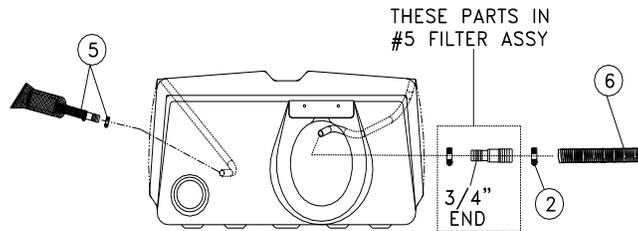
6. **Cut slot for Hose and Elbow Clearance:** Match tank to tank you have and cut slot as shown.
