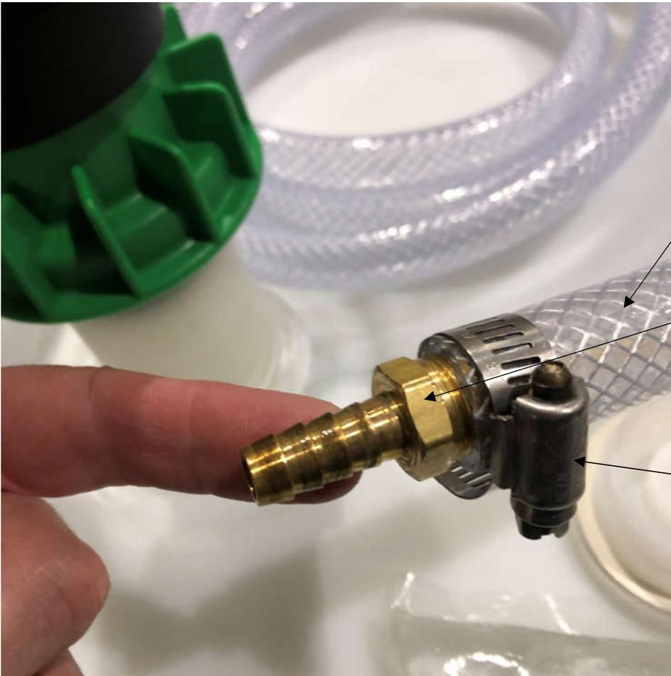
Attach a 2' long section of flexible vinyl hose to the Goat Throat Pump. Secure the hose to the pump using a worm drive hose clamp.
