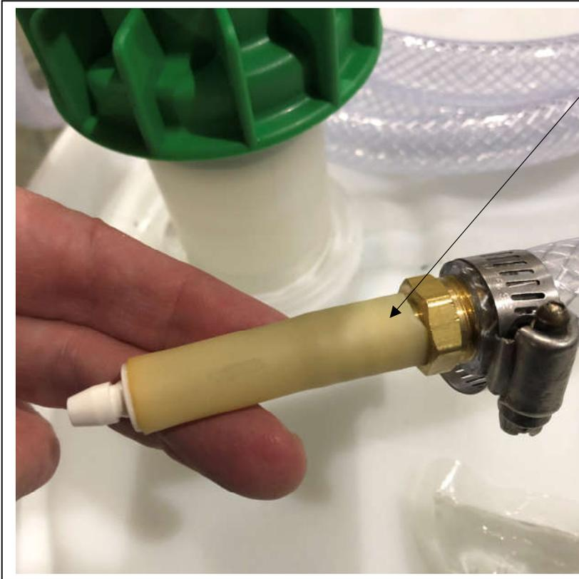
Slide the refill pump onto the brass hose barb. No clamp is needed but one can be used if desired.
