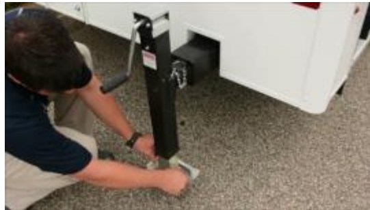
3. Remove Quick Adjust Pin.
