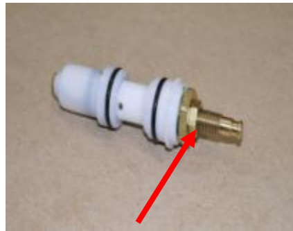
4. Adjust Cartridge by Loosening Hex Nut.
