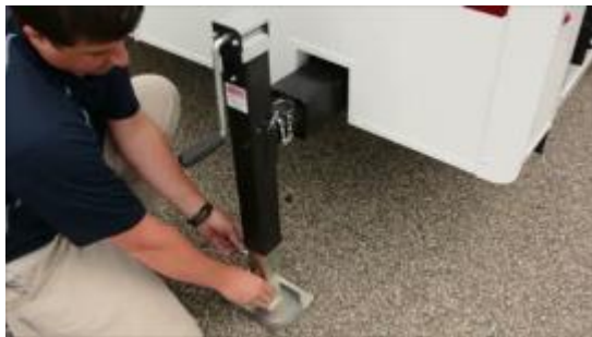
4. Adjust Height and Insert Pin.
