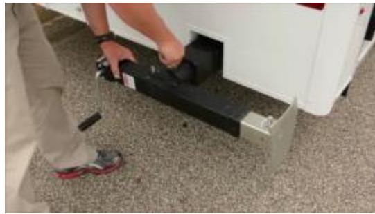
1. Remove Keeper Pin then rotate 90°.
