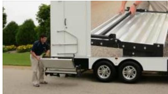
2. Pull Steps Out and Lock in Place With Spring Loaded Pins
