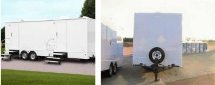
On site, first unhook from tow vehicle. Position the trailer on as level a surface as possible with the cabin doors facing the event. Always chock the trailer wheels. Position the sidewinder jacks, and use them to level it. Do not lift the tires off the ground. This can be done visually or with a level. Remember leveling the trailer side to side downhill will require you to support the downhill tires with a 2 X 8 boards or similar support.
