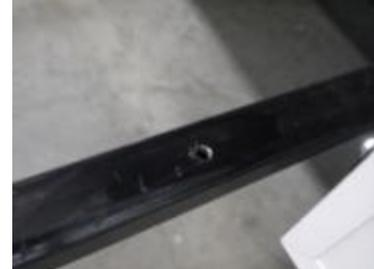
4. Lift Bracket and Pull Steps towards Trailer until Pin is Inserted into Lock Hole on Step Frame.
